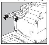
Re-fit the bottom panel using the 4 screws supplied with the door hinges (in the plastic bag) and the previously removed screw.
